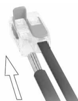
Installation of quick-connection blocks
